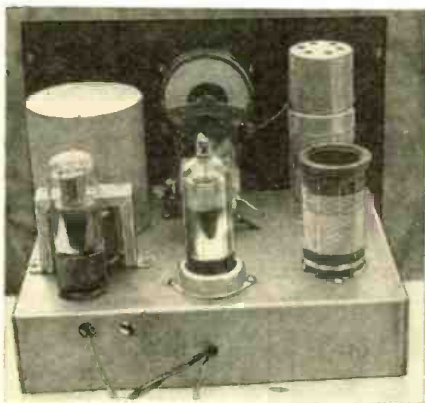
Rear view of the "Economy 3" Receiver—an extremely smooth-working set using the new 1.4 volt battery tubes. The 3 tubes will operate on a single dry cell "A" battery.
